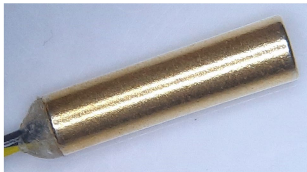
Figure 4. Inspection of the magnet under the microscope showing no evidence of erosion by gastric content.
