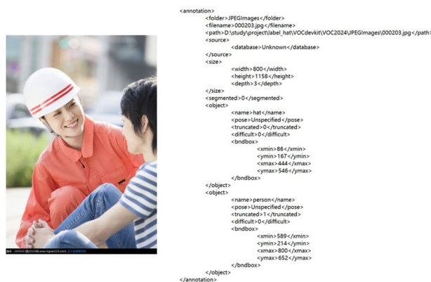
(a) Images used for training (b) xml annotation information for the image
