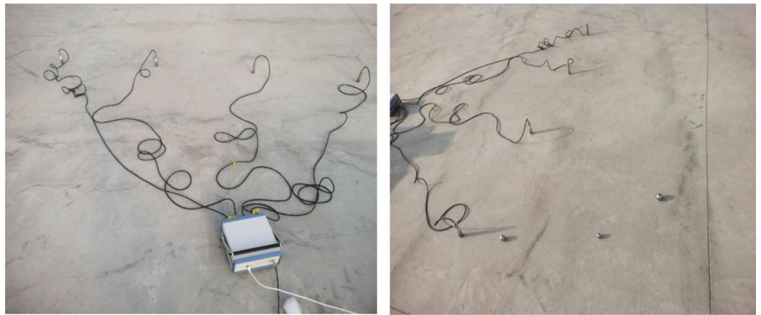
Figure 18. Diagram of sensor monitoring horizontal ground energy dissipation experiment.
