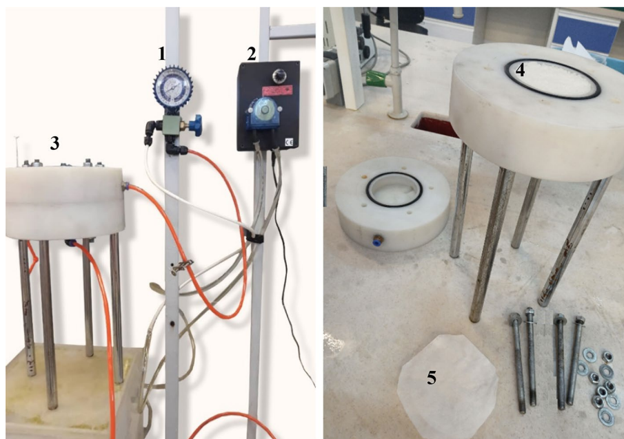
Figure 2. Schematic of the device for measuring the amount of passing NaCl solution. 1—Pressure gauge, 2—peristaltic pump, 3—Teflon water permeability system, 4—polypropylene granules, 5—mesh nets.
