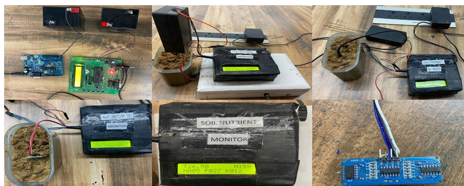
Figure 1. Working prototype for testing soil fertility.
