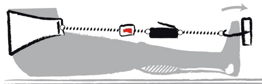
Figure 1. The mobile training system consisted of a kite-surfing harness, load scale, adjustable ratchet strap, and a stirrup. The scale provided instant feedback on the force applied to the stirrup during the isometric plantarflexion for the participants to adjust to the targeted intensity of the protocol. The length of the ratchet strap was adjusted so that an ankle angle of \sim 0^\circ (i.e., sole perpendicular to the shank) was achieved during the plateau of the contraction.
