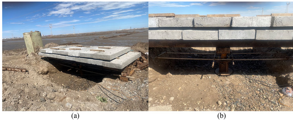
Figure 23. The schematic diagram of in-situ load tests: (a) Test device arrangement; (b) Apply load to the subsoil.
