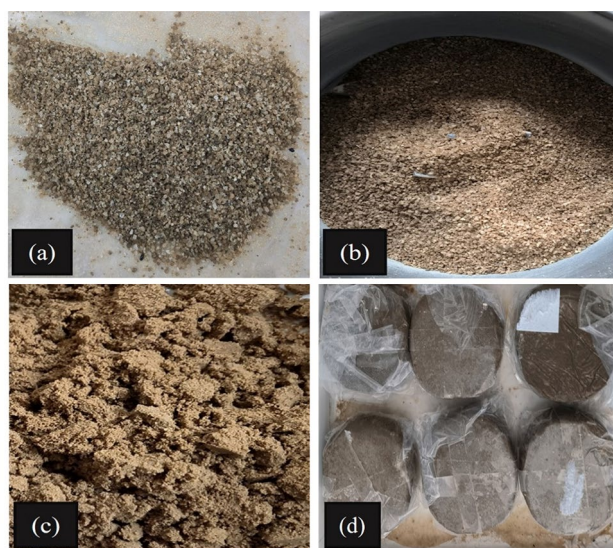
Figure 3. The process of sample preparation: (a) Drying natural saline soil; (b) Crushing natural saline soil; (c) humidifying natural saline soil; (d) Sample preparation and package.
