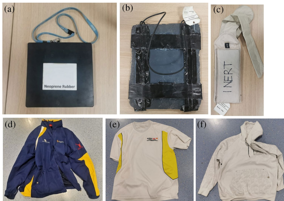
Figure 1. Photographs of simulated concealed weapons including (a) neoprene rubber block, (b) metal bearings in clay, and (c) fragments in money bag. Examples of outer clothing such as (d) layered windproof, (e) t-shirt, and (f) hoodie.
