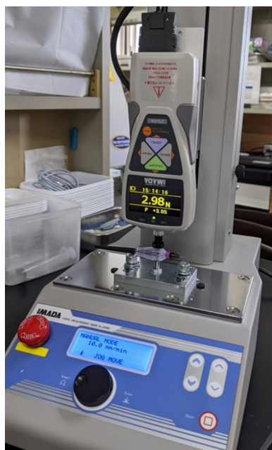
Figure 2. Measurement of the force required to close the forceps tips. The force is measured using a digital force gauge and a motorized test stand. The grips of the forceps are attached to a stand and pressed at a speed of 10 mm/min until the tips close.
