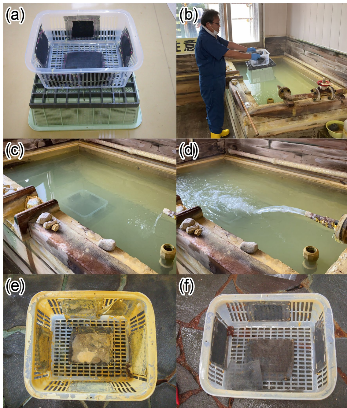
Figure 1. In situ Au adsorption experiment. (a) Blue-green algal sheets were attached to the bottom and sides of a PFA basket (30 cm by 25 cm by 15 cm high). Then, the PFA basket was set on an overturned plastic basket to prevent the blue-green algal sheets from being buried under hot spring water precipitate (sinter deposits). To prevent corrosion and contamination, no metal pieces were used. (b–d) Photographs taken (b) just before and (c, d) after the blue-green algal sheets and PFA basket were put into the test water tank at the Neutralisation Treatment Facility at Tamagawa Hot Spring. Hot spring water with a temperature of 60 °C and a pH of 1.2 flowed through the tank at a rate of 6 m 3 /h. (e) The blue-green algal sheets after the 7-month in situ Au adsorption experiment in the test water tank. The yellowish precipitate is a sinter deposit dominated by native sulfur. (f) The blue-green algal sheets just after they were washed with tap water to remove the sinter deposit.
