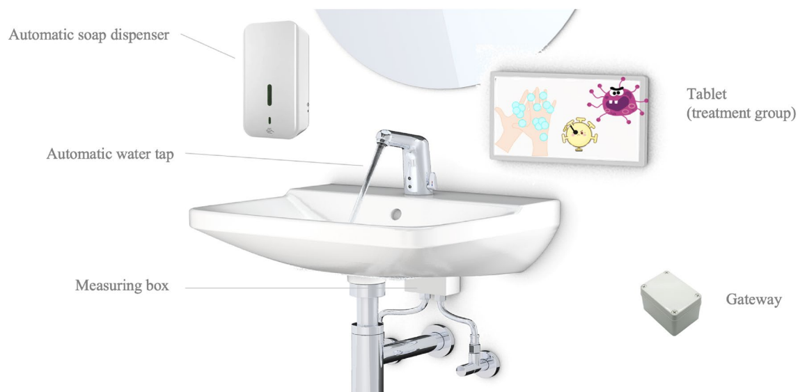
Figure 2. Schematic installation of the digital intervention at one washbasin, including an automatic.
