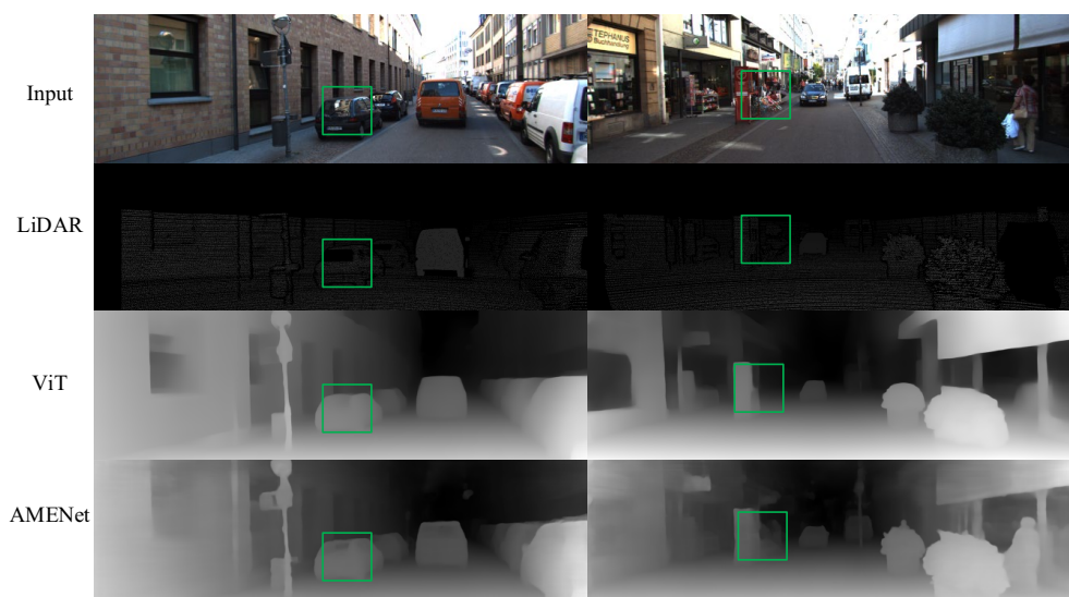
Figure 7. The test results on KITTI, the green boxes showcase that the proposed model handles details with minimal deviation from LiDAR measurements.
