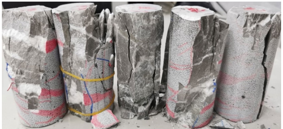
Figure 15. Damage state of all specimens after uniaxial test.
