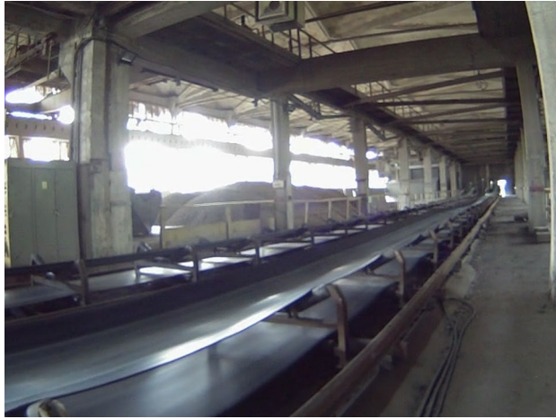
Figure 7. A general picture of the raw materials storage with BC to transport raw materials.
