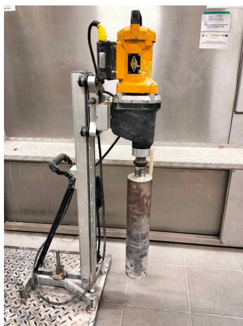
Figure 1. View and diagram of a hydraulic drilling rig used to collect samples (1—crown drill bit with a diameter of 100 mm; 2—ramp plate; 3—hydraulic power sockets, 4—bracket). (Own elaboration).
