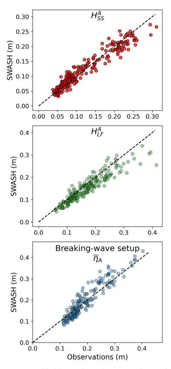
**Figure 4.** Model validation at the nearshore (sensor A) location of sea-swell significant wave height, low-frequency significant wave height, and breaking-wave setup.
