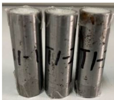
Figure 1. Glass microsphere-filled steel tube (GMFST) columns.
