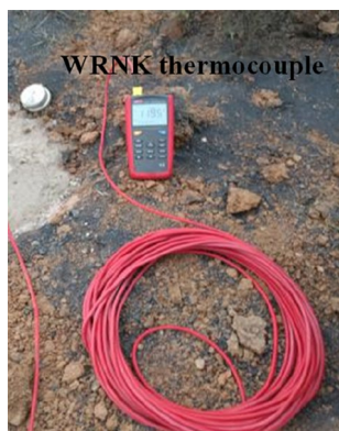
Figure 12. Temperature of the borehole measured by the WRNK thermocouple.
