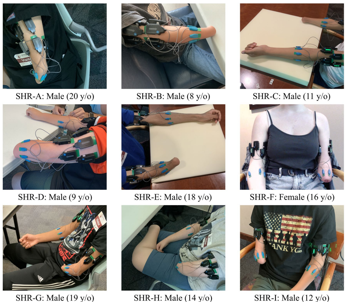
Figure 1. Participants with sEMG electrodes donned across unaffected and affected limbs with sex and age in years old (y/o) specified.
