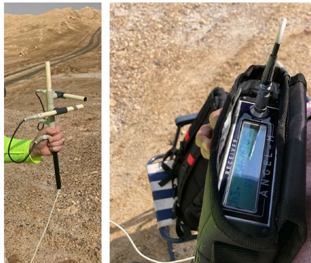
Figure 3. The photographs of the 3D antenna and Angel-M instrument during measurements at the Dead Sea region.
