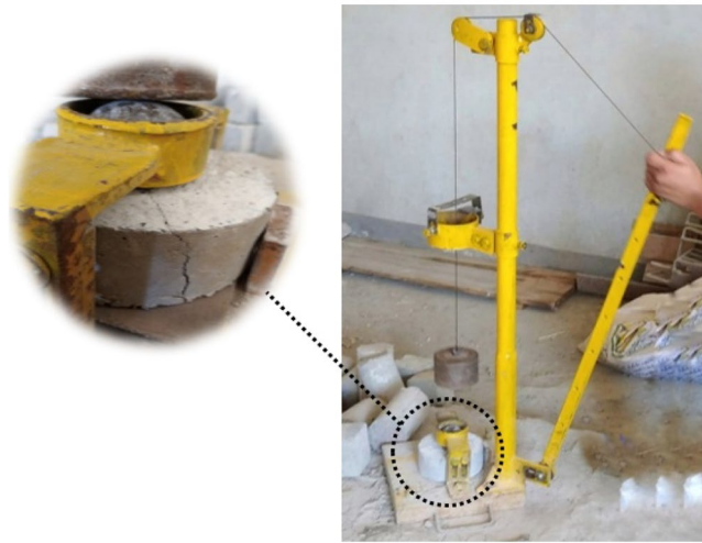
Figure 6. Impact test setup.
