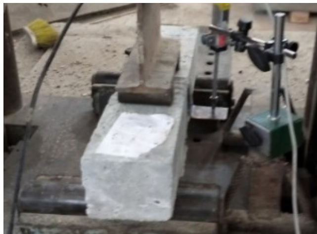
Figure 5. Flexure test setup.
