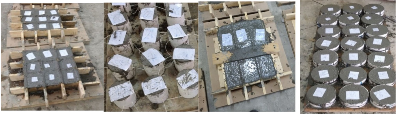
Figure 4. Compression, indirect tension, flexural, and impact specimens after casting.
