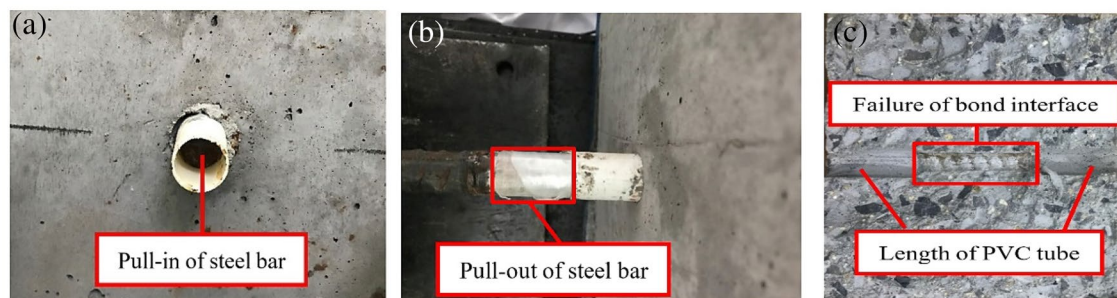
Figure 7. Typical failure patterns of tested specimens. (a) pull-in at free end (b) pull-out at tension end (c) failure surface on bond length.
