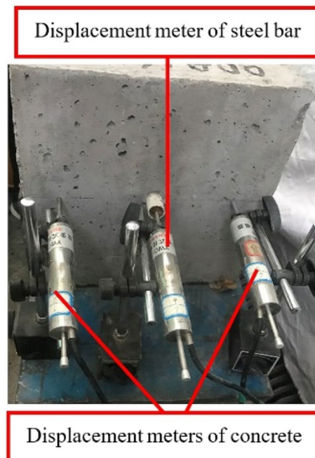
Figure 6. Displacement meters arrangement at free end of steel bar and on the surface of block.
