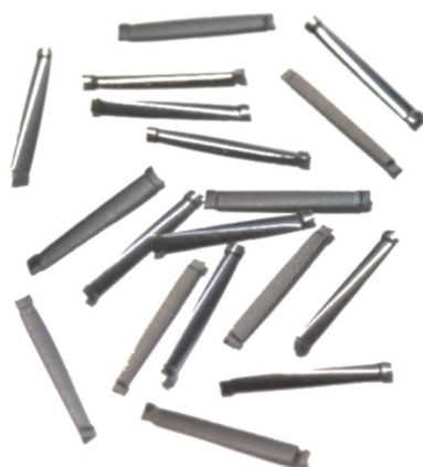
Figure 1. Ingot mill steel fibres used in this study.
