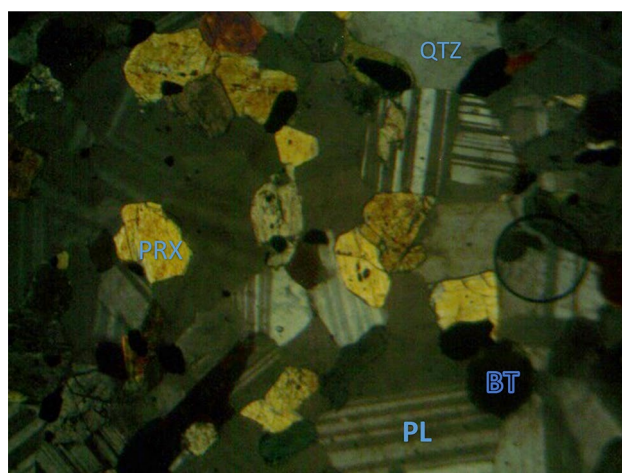
Figure 8. Microphotograph of charnockite (QTZ = quartz, PRX = Pyroxene, PL = Plagioclase and BT = B = Biotite).
