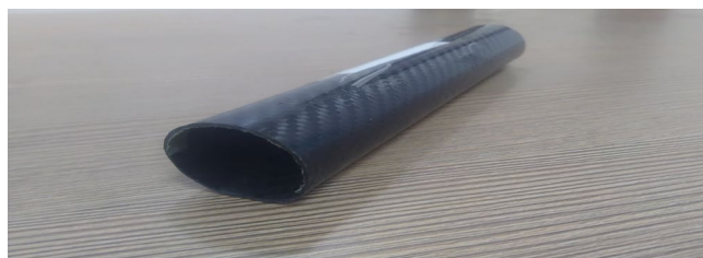
Figure 21. A typical view of test specimen before structural failure made of CFRP composite.
