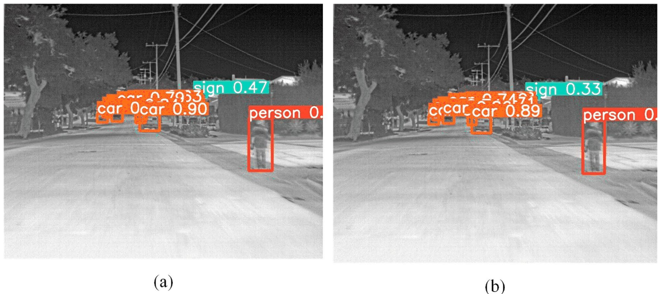
Figure 10. The detection results of our proposed algorithm and baseline network in infrared images. Due to the limitations of two-dimensional display, (a) represents the detection results of our proposed algorithm, including 1 person, 12 cars, and 1 sign; (b) represents the detection results of baseline network, including 1 person, 10 cars, and 1 sign.
