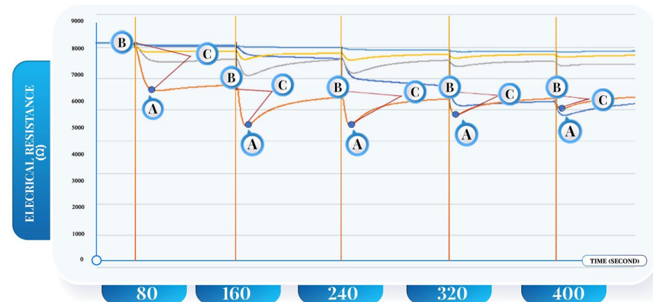
Figure 1. the Gas Sensor Analysis from the change of the electrical resistance in each sensor: Label sensor 2 (orange line) A = min or the lowest point of the electrical resistance of the voltage heater in each time which had five values min1- min5, C = the slope of the graph from plotting the time against the decrease of the electrical resistance. The C (the highest to the lowest) in each time had 5 values which were sl1-sl5. The delta resistance from point B to point A was equal to gap which had 5 values: gap1-gap5, time from B to A was equal to t which had 5 values (t1-t5). Abbreviation: \Omega = ohm; the unit of electrical resistance, sec = second, S = sensor (S1 = sensor No.1, S2 = sensor No.2,....., S5 = sensor No.5).
