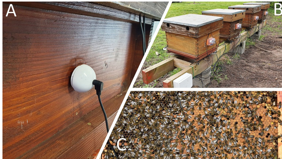
Figure 2. (A) Photo of the electromagnetic shaker (without protective box) secured to the outer wall of the brood box of the indoor hive, for the pilot study. (B) photo of a collection of four honeybee hives in Gent, Belgium, equipped with the same electromagnetic shakers, in individual weatherproof boxes. (C) photo of one side of the central frame of a honeybee hive equipped with an accelerometer inserted in the middle of the honeycomb. Although the black wire reveals the presence and the location of the accelerometer, the sensor itself is not visible anymore, as bees have built cells around it and are using them normally for brood, honey and bee-bread storage.
