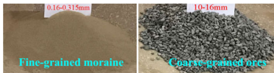
Figure 4. Test media of fine-grained moraine and coarse-grained ore.
