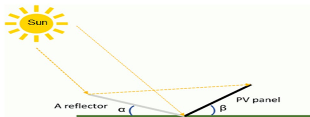
Figure 2. A schematic diagram for a PV with a reflector 19 .
