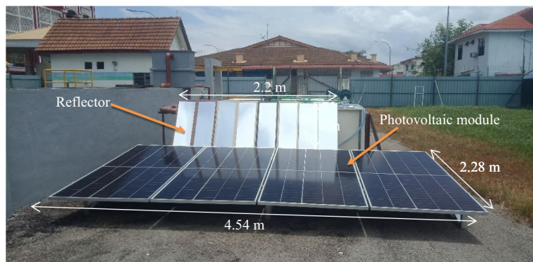
Figure 4. The experimental set up for the PV with a reflector.
