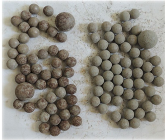
Figure 3. Grinding balls with \Phi 12 mm and \Phi 25 mm.
