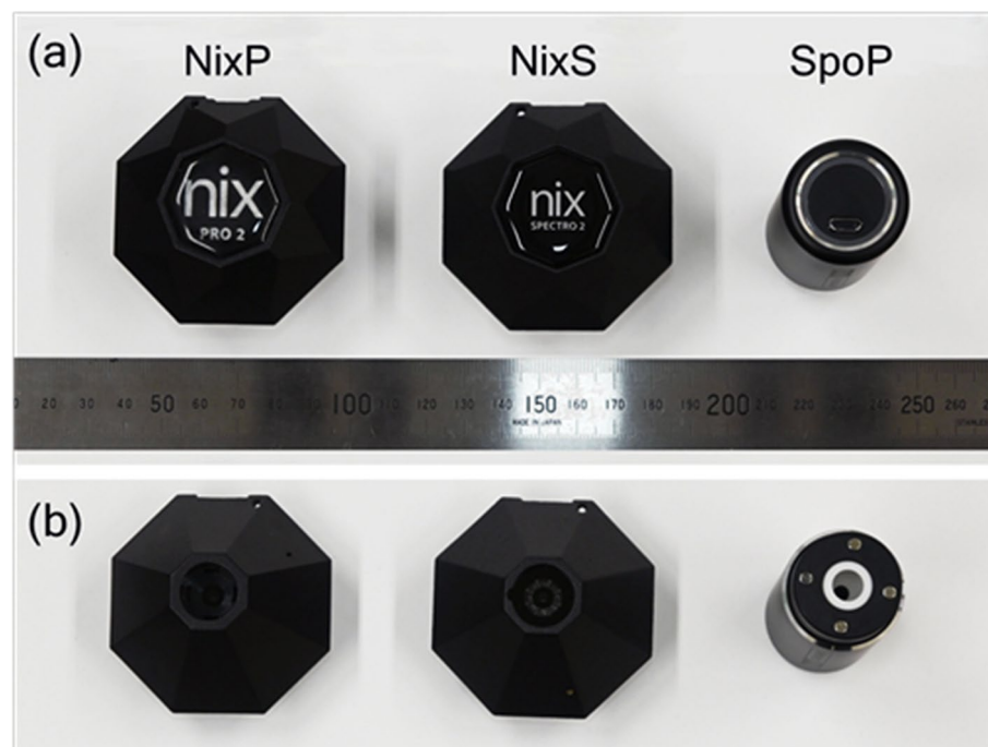
Figure 1. The sensors of three portable colorimeters employed in the present study. From the left, nix pro 2 (Nix Sensor Ltd.; abbreviated to “NixP”), nix spectro 2 (Nix Sensor Ltd.; “NixS”), and Spectro 1 Pro (Variable Inc.; “SpoP”). The upper photograph (a) was taken from the above and the lower one (b) taken from the bottom.
