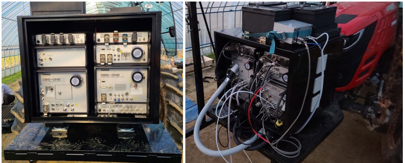
Figure 2. Portable emissions measurement system attached to the front part of the tractor.
