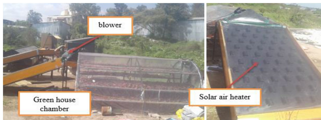
Figure 1. Mixed-mode solar red pepper dryer.
