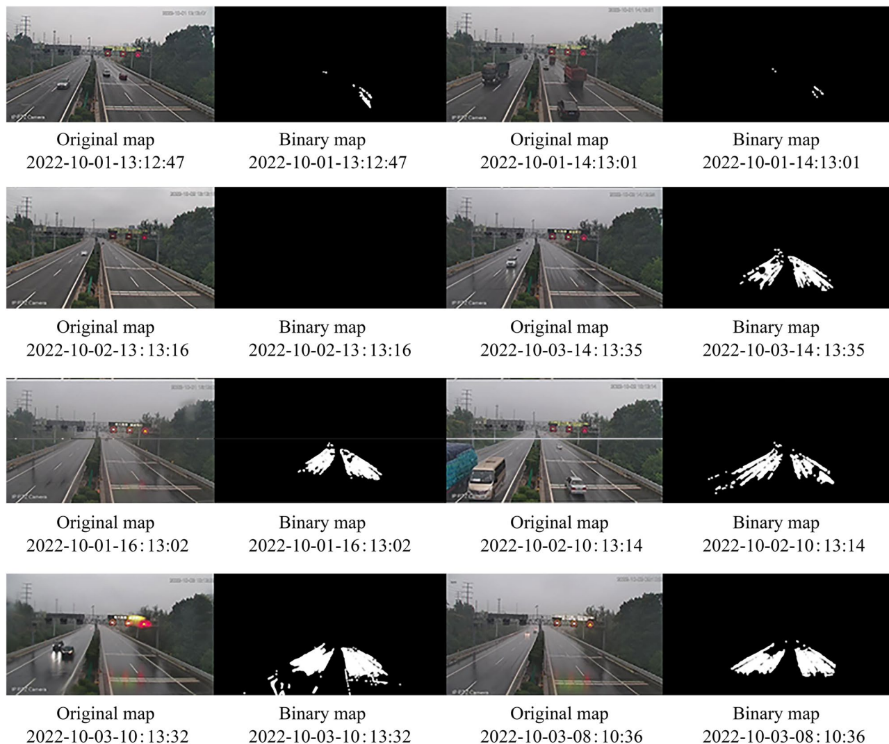
Figure 5. Data validation of Camera at K15+0.10 km of Jinan Ring Expressway G2001 Line in different time periods. The above image shows the original and processed binary images of the camera at K15+0.10 km of Jinan Ring Expressway G2001 at different time periods.
