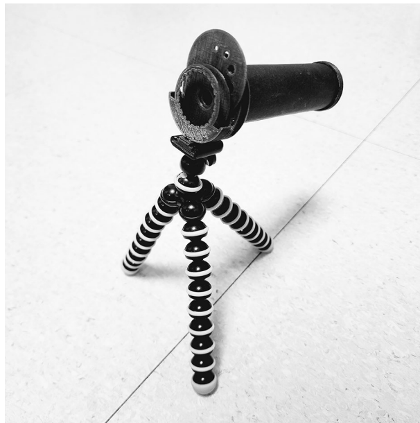
Figure 5. 3D printed schematic eye. Trial lenses can be mounted on the front to achieve the desired refractive error, and a disc with holes of different sizes can be rotated to vary the size of the pupil. The body tube is 10 cm long and has a default refractive error of +10 D.
