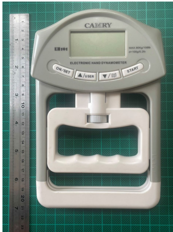
Figure 4. CAMRY digital hand dynamometer EH101 was used to measure the hand grip strength developed by each hand.
