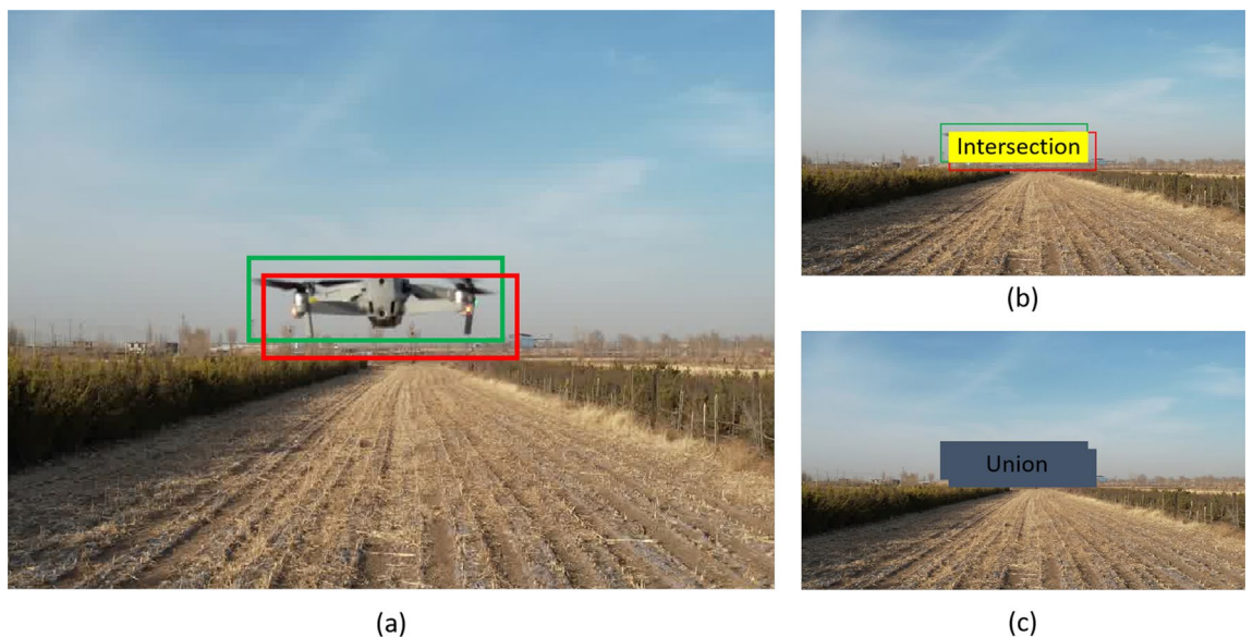
Figure 5. Intersection over Union (IoU) schematic diagram: (a) illustrates the positions of the predicted box and the ground truth box, (b) shows the intersection between the predicted box and the ground truth box, and (c) represents the union of the predicted box and the ground truth box.
