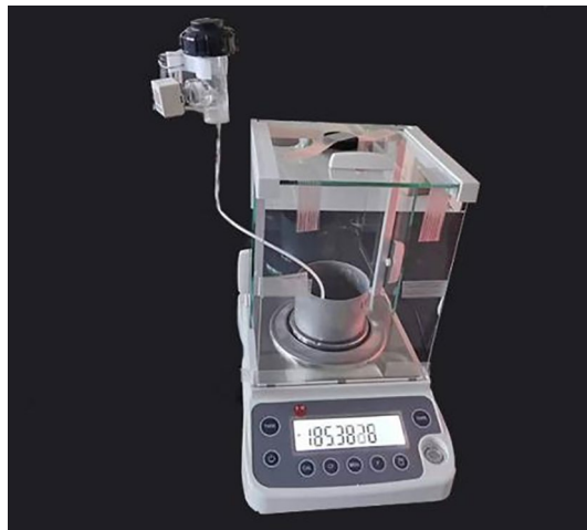
Figure 6. Test diagram of tensiometer method.
