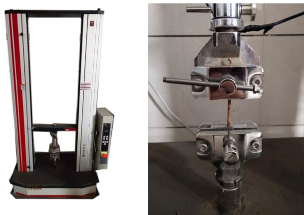
Figure 3. TY-8000 servo control testing machine and fixtures.
