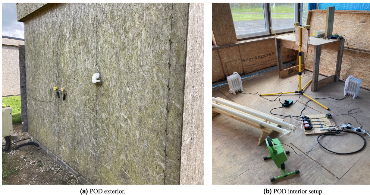
Figure 5. Set-up for the demonstration experiment, showing (a) the exterior of one POD and (b) the model appliance loads being controlled by the micro-controller and relays.
