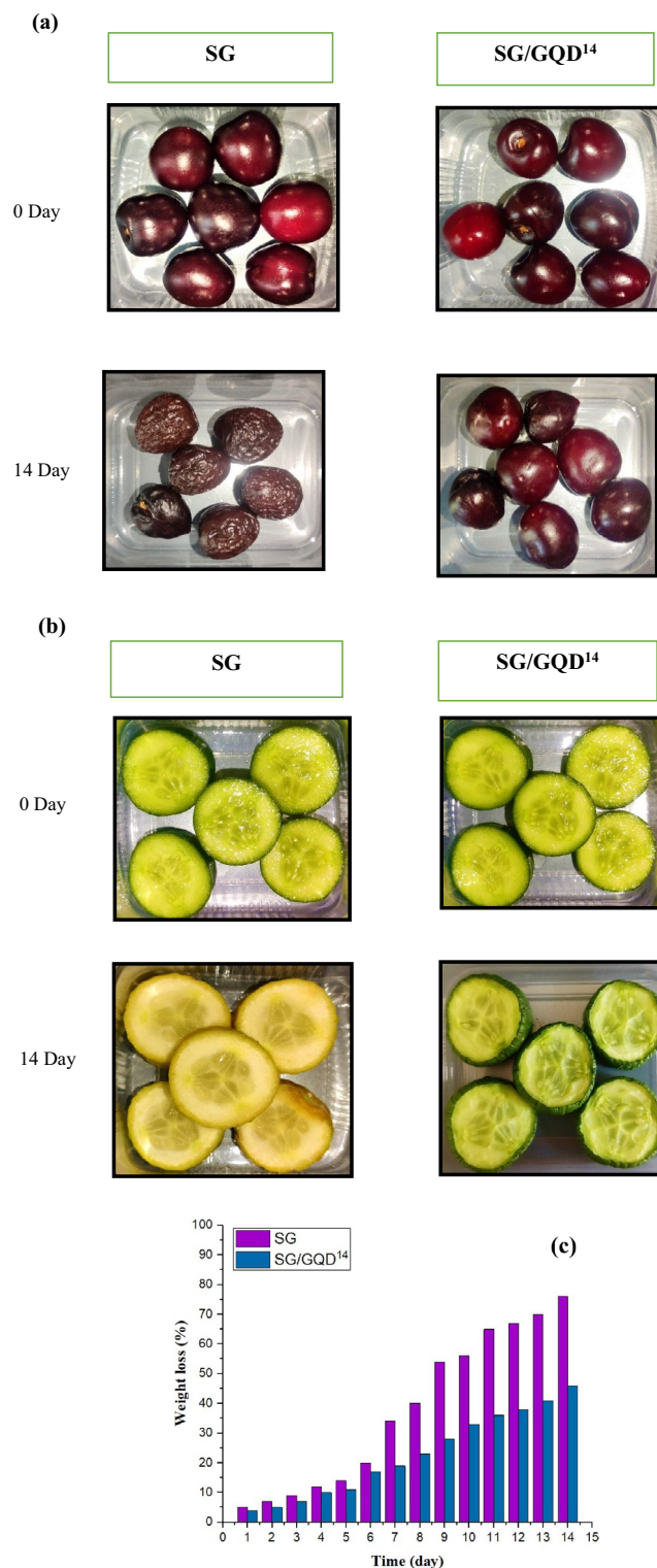
Figure 15. Protection test of cherries (a) and cucumbers weight losses of packaged fruits (b) (cherries (c) and cucumbers with and without GQDs (d).
