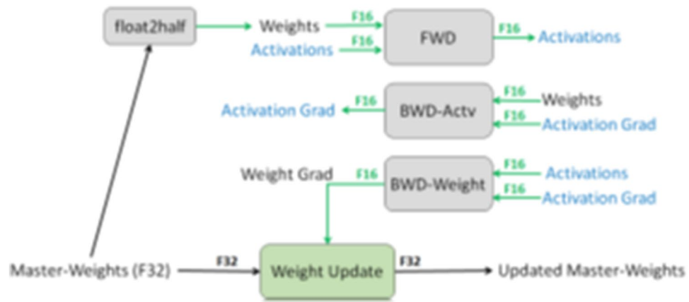
Figure 6. Mixed precision training iteration for a layer 83 .
