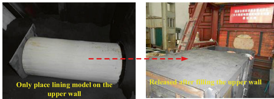
Figure 25. Comparative test of tunnel without crossing fault.
