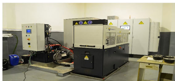
Figure 8. Gear contact fatigue testing machine.
