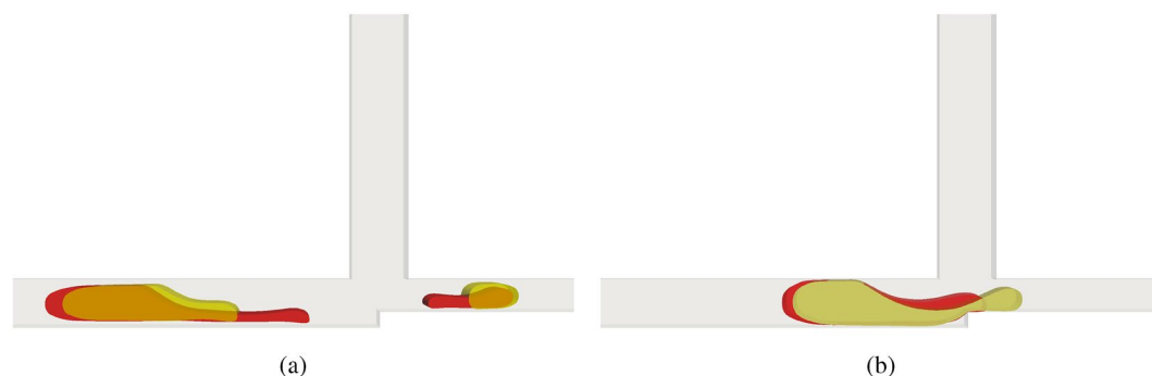
Figure 6. Influence of the Weissenberg number ( Wi ) for different capillary numbers of the viscoelastic fluid. The yellow fluid has Wi = 0.01 while the red fluid has Wi = 4 . Both fluids have Ca = 0.1 (a) and Ca = 0.01 (b).
