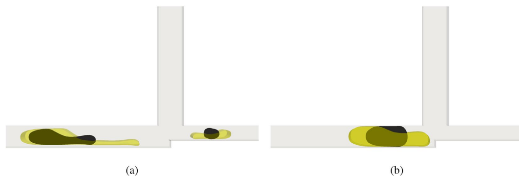
Figure 7. Comparison of the droplet initial size for the AND logic gate for Wi = 4 for ratios L/H equal to 2.4 (yellow droplet) and 1.4 (black droplet) for Ca = 0.1 .
