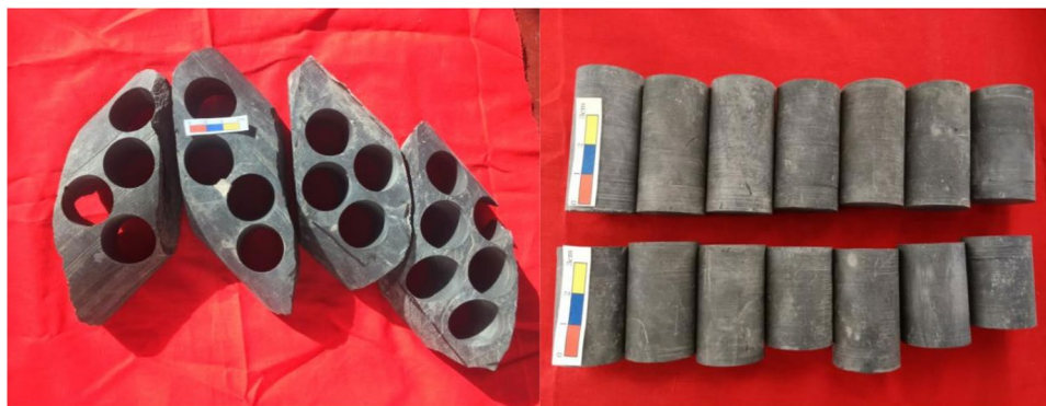
Figure 1. The original core samples and drilling core cylindrical samples with a 25 mm diameter.
