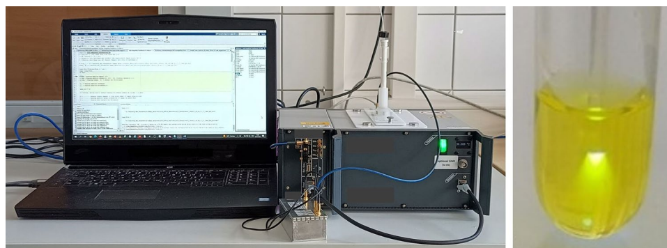
Figure 8. Experimental setup. Left image: Tabletop MRI with magnet, controller, small preamplifier and laptop. Right image: NMR tube with fiber positioned in pure \text{H}_2\text{O} containing FMN and favipiravir.
