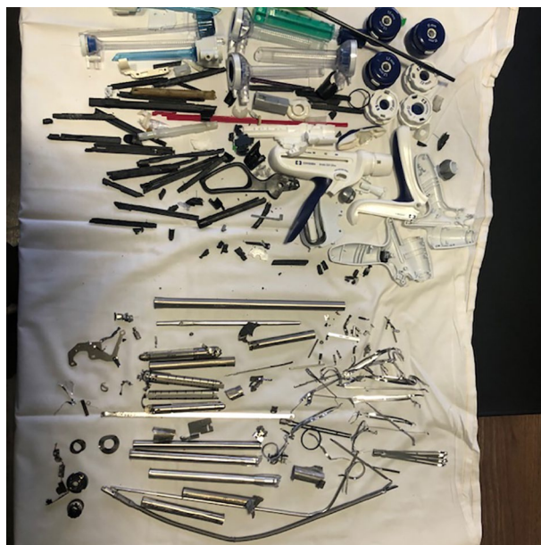
Figure 2. Separation of plastic parts and metallic parts, it may be published under a CC BY open access license.
