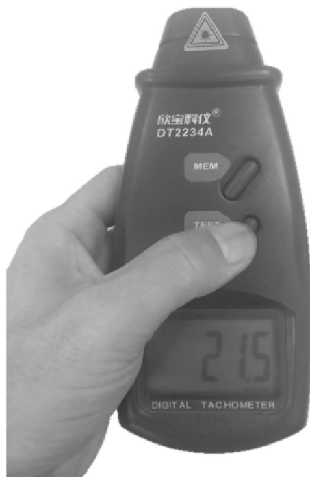
Figure 11. SM2234A non-contact tachometer.
