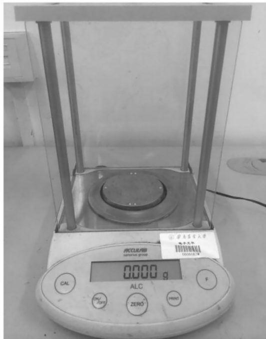
Figure 10. ALC-210.3 electronic balance.
