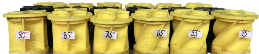
Figure 12. Groove wheels formed by 3D printing.
