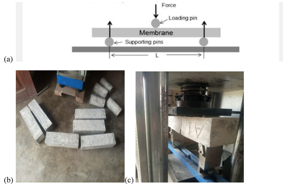
Figure 2. (a) Flexural strength test setup with the test sample for three-point test, (b) beams ready for testing, (c) beam testing by three-point test method.
