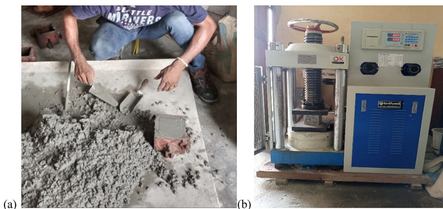
Figure 1. (a) Mixing and filling the cubic mold, (b) cube testing for compressive strength.
